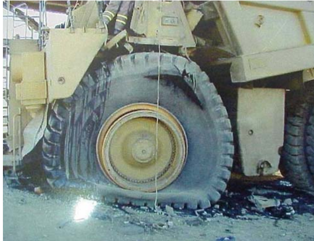
Figure 2.3.1 – Result of tire zipper failure [21].
